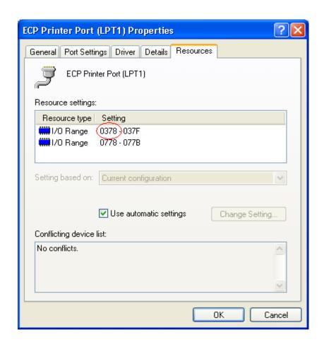
For many adapters the port address is shown under the resources of the Multi-IO adapter and not under LPT ports.
