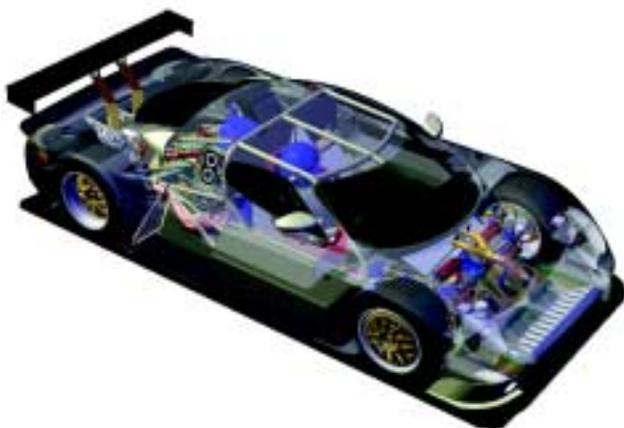
The Daytona Prototype built by FABCAR, demonstrated flawless performance during its maiden win in the Nextel Grand Prix of Miami in March 2003. Designed in Solid Edge and analyzed suspension and roll bar using CAEFEM by Fin-el, LLC.
